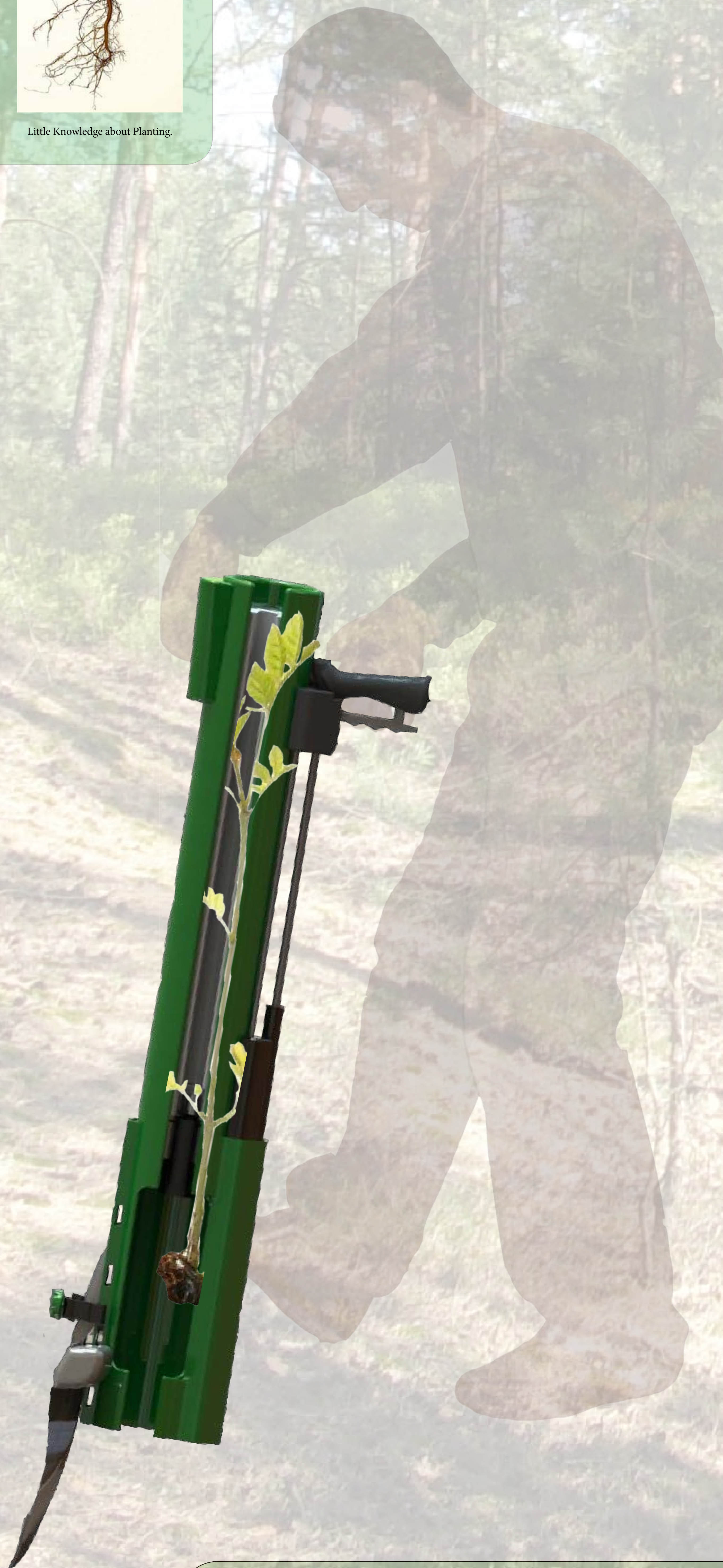
The Catch Mechanism opens up and the sapling root is caught just over the Root Collar of the Tree Sapling.
