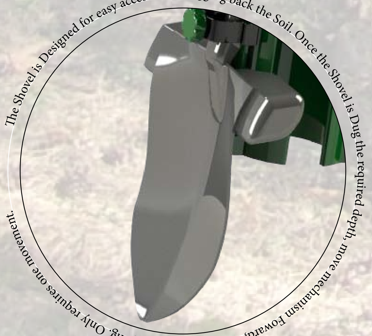
Lock Mechanism when Released can Adjust the depth of cut for the shovel which is adjust for different sized Tree Saplings.
