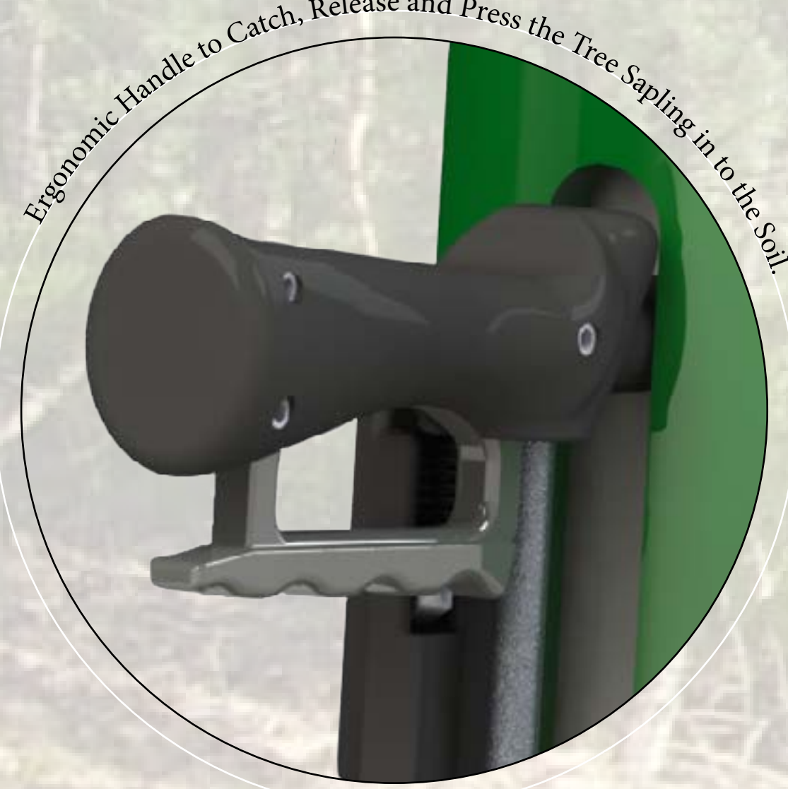
The Catch Mechanism opens up and the sapling root is caught just over the Root Collar of the Tree Sapling.
